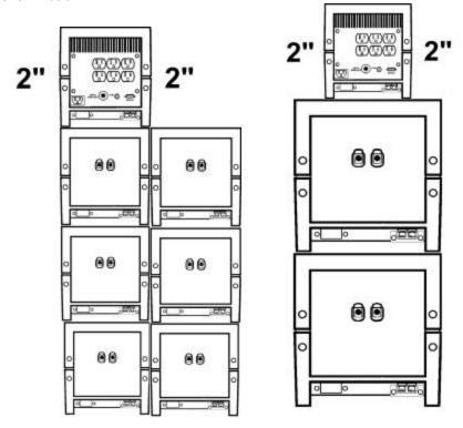
Remember to leave at least 2 inches of clearance around the UPS unit for air flow.
